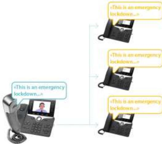
You can broadcast emergency messages in real-time mode through Cisco IP phones. Just push a button on any IP phone, enter the PIN to authorize and start speaking!
